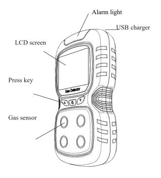
2.2 Working principle Electrochemical and catalytic combustion
